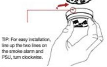
**OPTION 2: ALARM MOUNTED ON TOP OF** CONDUIT BOX:
