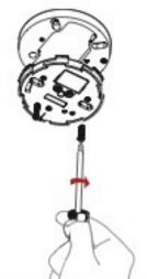
Once the mounting base with power supply unit is installed, attach the alarm by twisting clockwise until it clicks. If the battery is either missing or inserted incorrectly, the smoke alarm will not be able to click into the mounting base.
