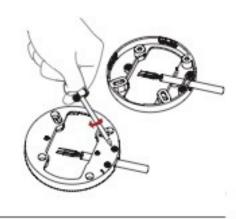
Connect the 3 wires to the power supply unit: Live feed (L1), neutral (N), Ground ( $\pm$ ).
