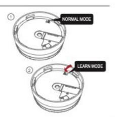
Please note: The learn switch placed on the back of the alarm can only be in learn position when the alarm is disassembled from the power supply unit. The learn switch will automatically switch to normal position when the alarm head is fitted to the power supply unit.
