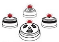
When all alarms flash the red LED, they are connected and can be switched out of 'Learn Mode' and installed.
