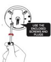
Screw the power supply unit on the mounting base.
